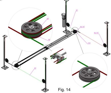
Note: If Cable(s) comes off the Cable Sheave, it will be required to remove the Cable Sheave assembly to reinstall the Cable, due to welded cable guide brackets.
